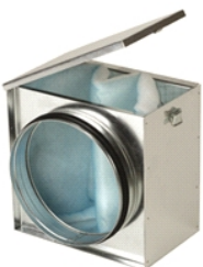
MFL filtration boxes are of G4 grade filtration and are designed for direct connection with standard circular ducting. The MFL-G4 filtration boxes are supplied with a cover easily removable to replace the filter.
